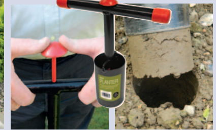
Bulb Planters When planting bulbs in the open ground simply push the planter into the ground, twist 3 or 4 times. Remove and place bulb in the hole, press red plunger to eject soil back into the hole. Bulb planting made easy! Heavy duty black powder coated for longer life. Can also be used as a potato planter. Hand bulb planter 46094 £18.00 Long handled planter 46095 £29.10
